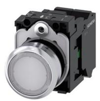
Illuminated pushbutton, 22 mm, round, metal, shiny, white, pushbutton, flat, momentary contact type, with holder, 1NO, LED module with integrated LED 24 V AC/DC, spring-type terminal, with laser labeling, lower case
