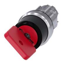
Key-operated switch O.M.R, 22 mm, round, metal, shiny, lock number 73037, red, with 2 keys, 2 switch positions O-I, latching, actuating angle 90°, 10:30h/13:30h, key removal O+I, with laser labeling, upper case and lower case, always upper case at the beginning of the word
