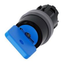
Key-operated switch O.M.R, 22 mm, round, plastic with metal front ring, lock number 73038, blue, with 2 keys, 2 switch positions O-I, latching, actuating angle  $90^\circ,\,10:\!30h/13:\!30h,$  key removal O, with laser labeling, upper case and lower case, always upper case at beginning of line
