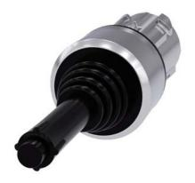
Coordinate switch, 22 mm, round, metal shiny, black, 4 switch positions, momentary contact type, with mechanical interlocking, Z=50-unit packaging
