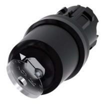
Key-operated switch IKON, 22 mm, round, plastic, lock number 360012K1, with 2 keys, 2 switch positions O-I, latching, actuating angle  $90^\circ$ , 10:30h/13:30h, key removal O, with laser labeling, upper case and lower case, always upper case at the beginning of the word
