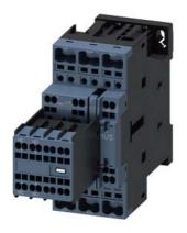
Contactor, AC-3, 15 kW / 400 V, 2 NO + 2 NC, 110 V AC, 50 / 60 Hz, 3-pole, Size S0, Spring-type terminal Removable auxiliary switch
