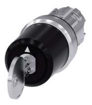
Key-operated switch BKS, 22 mm, round, metal, shiny, lock number S1, with 2 keys, 3 switch positions I-O<II, left latching, right momentary contact type, actuating angle 2x45°, 10:30h/12h/13:30h, key removal I, with laser labeling, upper case and lower case, always upper case at the beginning of the word
