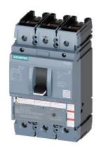
circuit breaker 3VA5 UL frame 250 breaking capacity class C 100kA @ 480 V 3-pole, line protection TM230, FTAM, In=80A overload protection Ir=80A fixed short-circuit protection Ii=5...10 x In cable connection on both sides
