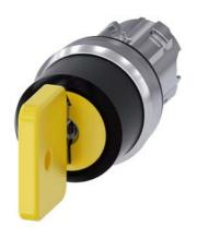
Key-operated switch O.M.R, 22 mm, round, metal, shiny, lock number 73033, yellow, with 2 keys, 3 switch positions I>O<II, momentary contact on the left, latching on the right, actuating angle  $2x45^{\circ}$ , 10:30h/12h/13:30h, Key removal II, Z=50-unit packaging
