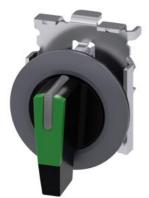
Selector switch, illuminable, 30 mm, round, Metal, matte, green, selector switch, long, front ring for flush installation, 3 switch positions I-O-II, latching, actuating angle 2x45°, 10:30h/12h/13:30h, with laser labeling, lower case
