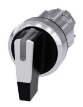
Selector switch, illuminable, 22 mm, round, metal, shiny, white, selector switch, long, 3 switch positions I-O-II, latching, actuating angle 2x45°, 10:30h/12h/13:30h, Z=50-unit packaging
