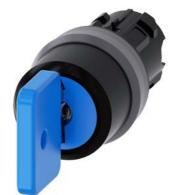
Key-operated switch O.M.R, 22 mm, round, plastic with metal front ring, lock number 73038, blue, with 2 keys, 3 switch positions I-O-II, latching, actuating angle 2x45°, 10:30h/12h/13:30h, Key removal I+O+II, with laser labeling, upper case
