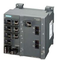
SCALANCE X308-2, managed plus IE switch, 2x 1000 Mbit/s MM SC 1x 10/100/1000 Mbit/s and 7x 10/100 Mbit/s RJ45 ports, LED diagnostics, error signaling contact with select/set pushbutton, PROFINET IO device, network management, integrated redundancy manager, office features (RSTP, VLAN, IGMP,..) C-PLUG in scope of supply.
