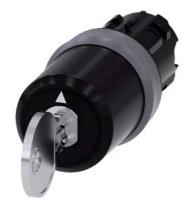
Key-operated switch BKS, 22 mm, round, plastic with metal front ring, lock No. E9 (VW), without key, 3 switch positions I-O-II, latching, actuating angle 2x45°, 10:30h/12h/13:30h, Key removal I+O+II, with laser labeling, upper case
