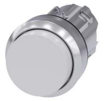
Pushbutton, 22 mm, round, metal, shiny, white, pushbutton, raised momentary contact type, with laser labeling, upper case and lower case, always upper case at beginning of line
