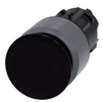
Mushroom pushbutton, 22 mm, round, plastic with metal front ring, black, 30 mm, latching, pull-to-unlatch mechanism, with laser labeling, upper case and lower case, always upper case at beginning of line
