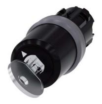
key-operated switch Siemens, 22 mm, round, plastic with metal front ring, special lock, with 2 keys, 2 switch positions O<I, momentary contact type, actuating angle  $45^\circ,\,10:30h/12h,$  key removal O
