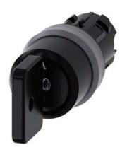
Key-operated switch O.M.R, 22 mm, round, plastic with metal front ring, lock number 73034, black, with 2 keys, 3 switch positions I-O-II, latching, actuating angle 2x45°, 10:30h/12h/13:30h, key removal O, with laser labeling, upper case
