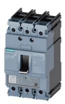
circuit breaker 3VA5 UL frame 125 3-pole, starter protection TM120M, AM, In=70A without overload protection short-circuit protection li=5...12 x In cable connection on both sides
