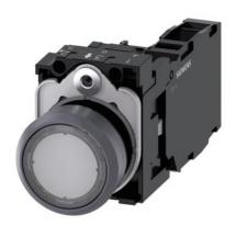
Illuminated pushbutton, 22 mm, round, plastic with metal front ring, clear, pushbutton, flat, momentary contact type, with holder, 1 NO+1 NC, LED module with integrated LED 230 V AC, screw terminal, with laser labeling, upper case and lower case, always upper case at beginning of line
