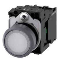
Illuminated pushbutton, 22 mm, round, plastic with metal front ring, white, pushbutton, flat, momentary contact type, with holder, 1NO, LED module with integrated LED 110 V AC, screw terminal, Z=20-unit packaging
