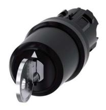
Key-operated switch IKON, 22 mm, round, plastic, lock number 360012K1, with 2 keys, 3 switch positions I-O-II, latching, actuating angle 2x45°, 10:30h/12h/13:30h, Key removal I+O+II, with laser labeling, upper case
