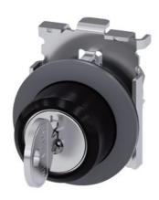
RONIS key-operated switch, 30 mm, round, Metal, matte, front ring for flush installation, lock number SB30, with 2 keys, 3 switch positions I-O-II, latching, actuating angle 2x45°, 10:30h/12h/13:30h, Key removal I+O+II, possible special locks: SB31, 421, 455, with laser labeling, inscription or symbol Customer-specific selection with SIRIUS ACT configurator (CIN)
