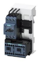
Fuseless motor starter Reversing operation 600VAC Size S00 0.11-0.16a 110/120VAC 50/60HZ screw connection For snapping onto 60 mm busbar systems Type of coordination 2 IQ = 150 KA Also full fills type Of coordination 1 1NC (per contactor)
