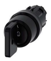
Key-operated switch O.M.R, 22 mm, round, plastic, lock number 73034, black, with 2 keys, 3 switch positions I-O<II, left latching, right momentary contact type, actuating angle 2x45°, 10:30h/12h/13:30h, key removal I, with laser labeling, lower case
