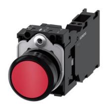
Pushbutton, 22 mm, round, plastic, red, pushbutton, flat, momentary contact type, with holder 1 NO+1 NC, spring-type terminal, with laser labeling, symbol number according to, ISO 7000 or IEC 60417
