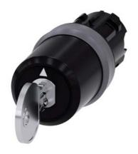
Key-operated switch BKS, 22 mm, round, plastic with metal front ring, lock number S1, with 2 keys, 3 switch positions I>O<II, momentary contact type, actuating angle 2x45°, 10:30h/12h/13:30h, key removal O, with laser labeling, upper case
