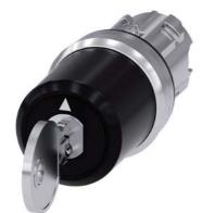
Key-operated switch BKS, 22 mm, round, metal, shiny, lock number S1, with 2 keys, 3 switch positions I-O<II, left latching, right momentary contact type, actuating angle 2x45°, 10:30h/12h/13:30h, key removal I, with laser labeling, upper case
