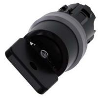
Key-operated switch O.M.R, 22 mm, round, plastic with metal front ring, lock number 73034, black, with 2 keys, 2 switch positions O-I, latching, actuating angle 90°, 10:30h/13:30h, key removal I, with laser labeling, inscription or symbol Customer-specific selection with SIRIUS ACT configurator (CIN)
