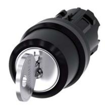
RONIS key-operated switch, 22 mm, round, plastic, lock number SB30, with 2 keys, 3 switch positions I-O-II, latching, actuating angle 2x45°, 10:30h/12h/13:30h, key removal O+I, possible special locks: SB31, 421, 455, with laser labeling, upper case
