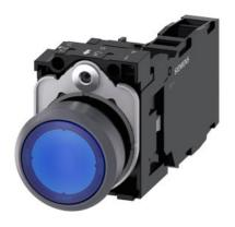
Illuminated pushbutton, 22 mm, round, plastic with metal front ring, blue, pushbutton, flat, momentary contact type, with holder, 1 NO+1 NC, LED module with integrated LED 110 V AC, screw terminal, with laser labeling, upper case and lower case, Always upper case at the beginning of the word
