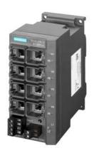
SCALANCE X108PoE unmanaged IE switch, 2x 10/100 Mbit/s RJ45 Power-over-Ethernet ports and 6x 10/100 Mbit/s RJ45 ports, LED diagnostics, error signaling contact with set pushbutton, redundant power supply manual available as a download .
