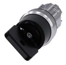
Key-operated switch O.M.R, 22 mm, round, metal, shiny, lock number 73034, black, with 2 keys, 2 switch positions O<I, momentary contact type, Actuating angle 45°, 10:30h/12h, key removal O, with laser labeling, upper case and lower case, always upper case at the beginning of the word
