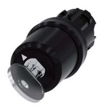
Key-operated switch BKS, 22 mm, round, plastic, lock number S1, with 2 keys, 2 switch positions O-I, latching, actuating angle  $90^\circ$ , 10:30h/13:30h, key removal O, with laser labeling, lower case
