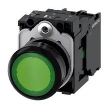
Illuminated pushbutton, 22 mm, round, plastic, green, pushbutton, flat, momentary contact type, with holder, 1NO, LED module with integrated LED 230 V AC, screw terminal, with laser labeling, inscription or symbol Customer-specific selection with SIRIUS ACT configurator (CIN)
