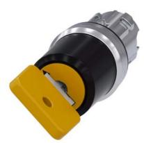
Key-operated switch O.M.R, 22 mm, round, metal, shiny, lock number 73033, yellow, with 2 keys, 2 switch positions O-I, latching, actuating angle 90°, 10:30h/13:30h, key removal O+I, with laser labeling, lower case
