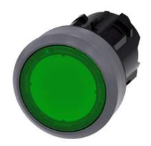
Illuminated pushbutton, 22 mm, round, plastic with metal front ring, green, pushbutton, flat, latching, Push-to-release mechanism, with laser labeling, upper case and lower case, Always upper case at the beginning of the word
