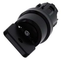
Key-operated switch O.M.R, 22 mm, round, plastic, lock number 73034, black, with 2 keys, 2 switch positions O<I, momentary contact type, Actuating angle 45°, 10:30h/12h, key removal O, with laser labeling, upper case and lower case, always upper case at the beginning of the word
