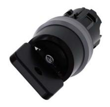
Key-operated switch O.M.R, 22 mm, round, plastic with metal front ring, lock number 73034, black, with 2 keys, 2 switch positions O-I, latching, actuating angle 90°, 10:30h/13:30h, key removal O+I, with laser labeling, upper case and lower case, always upper case at beginning of line
