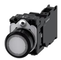
Illuminated pushbutton, 22 mm, round, plastic, clear, pushbutton, flat, momentary contact type, with holder, 1 NO+1 NC, LED module with integrated LED 110 V AC, spring-type terminal, with laser labeling, lower case
