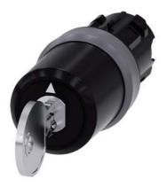
Key-operated switch BKS, 22 mm, round, plastic with metal front ring, special lock, with 2 keys, 3 switch positions I-O<II, latching on the left, momentary contact type on the right, actuating angle 2x45°, 10:30h/12h/13:30h, key removal O+I, Note: BKS locking systems E1 - E25 supplied without key
