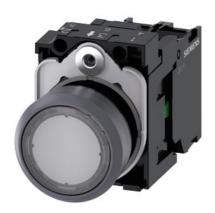
Illuminated pushbutton, 22 mm, round, plastic with metal front ring, clear, pushbutton, flat, momentary contact type, with holder, 1NO, LED module with integrated LED 230 V AC, screw terminal, with laser labeling, lower case
