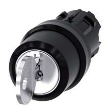
RONIS key-operated switch, 22 mm, round, plastic, lock number SB30, with 2 keys, 3 switch positions I-O-II, latching, actuating angle 2x45°, 10:30h/12h/13:30h, Key removal I+O+II, possible special locks: SB31, 421, 455, with laser labeling, inscription or symbol Customer-specific selection with SIRIUS ACT configurator (CIN)
