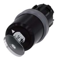
Key-operated switch BKS, 22 mm, round, plastic with metal front ring, lock No. E9 (VW), without key, 2 switch positions O-I, latching, actuating angle 90°, 10:30h/13:30h, key removal O, with laser labeling, inscription or symbol Customer-specific selection with SIRIUS ACT configurator (CIN)
