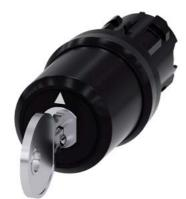
key-operated switch Siemens, 22 mm, round, plastic, lock number SSG10, with 2 keys, 3 switch positions I-O-II, latching, actuating angle 2x45°, 10:30h/12h/13:30h, key removal O+I, with laser labeling, inscription or symbol customer-specific selection with SIRIUS ACT configurator (CIN)
