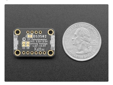
"OK, this thing sounds great. Give me some details" you say. OK then, here you go: The wiper value is a 7-bit number meaning there are 128 possible levels of resistance to choose, from 0-10K ohms. You can even set a default value that will be set on power up. The analog voltage controlled can be from 4.5-15.5V. Additionally you can use the address jumpers or pins to set the I2C address to one of four values, allowing you to have four DS3502s on the same I2C bus.
