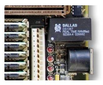
The image above shows a computer motherboard with a Real Time Clock called the  $\underline{D}$  S1387 (). There's a lithium battery in there which is why it's so big.
