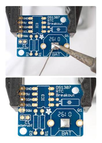
Begin by soldering a small bump onto the negative pad of the battery: this will make better contact!
