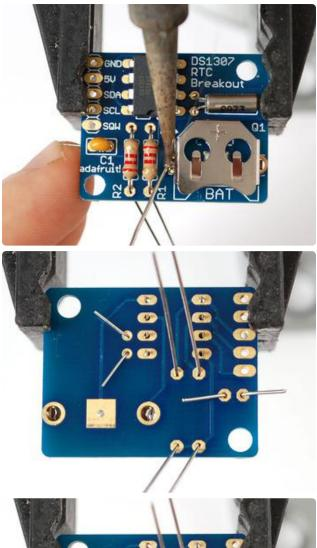
To keep the battery holder from falling out, you may want to 'tack' solder it from the top.
