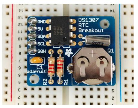
This is a great battery-backed real time clock (RTC) that allows your microcontroller project to keep track of time even if it is reprogrammed, or if the power is lost. Perfect for datalogging, clock-building, time stamping, timers and alarms, etc. The DS1307 is the most popular RTC, and works best with 5V-based chips such as the Arduino.
