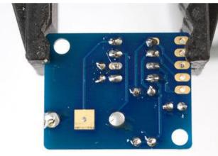
Clip the leads of the resistors, crystal and capacitor short.
