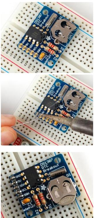
If you'd like to use the header to plug the breakout board into something, place the header in a breadboard, long side down and place the board so that the short pins stick thru the pads.
