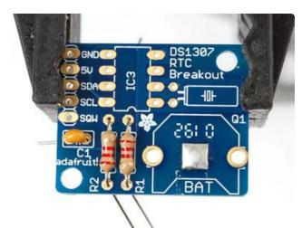
Place the two 2.2K resistors, and the ceramic capacitor. They are symmetric so no need to worry about direction. If you're planning on using with a Raspberry Pi (which has 3.3V logic and built in pull-ups, skip the 2.2K resistors!
