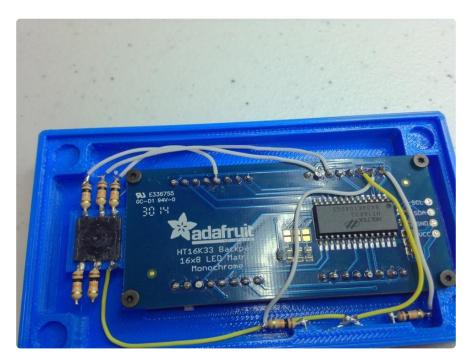
Solder a white wire to each of the resistors on the left side of the joystick, and make the connections shown in the picture above. If the picture looks confusing, please refer to the circuit diagram on the previous page.
