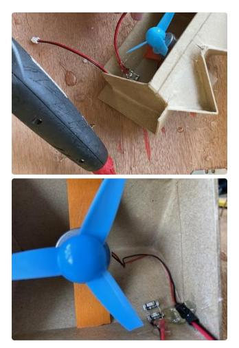
Using hot glue, secure the fan's cabling to the roof.
