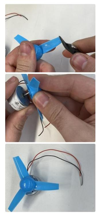
Modify the propeller by cutting ~0.4mm off each end of the propeller with a pair of scissors or wire cutters.
