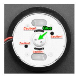
Apply a small dab of glue (or hot glue) to the back of the motor. We've marked on the image where the glue could leak into the motor.
