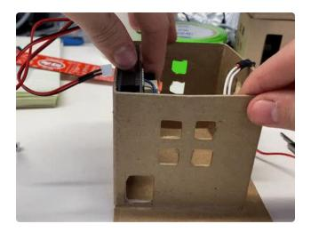
Connect up all the JST connectors and close the roof of the home.
