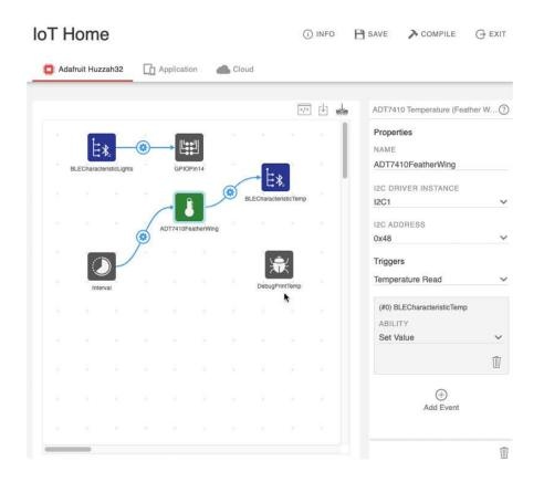
To summarize - every time the interval's timer expires, the ADT7410 will read the temperature. Once the temperature is read from the sensor, it'll be sent to the BLECharacteristicTemp element and printed to the UART console.
