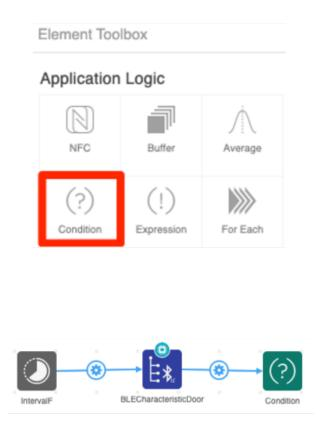
To evaluate if the door is open or closed, a comparison element needs to be added.
