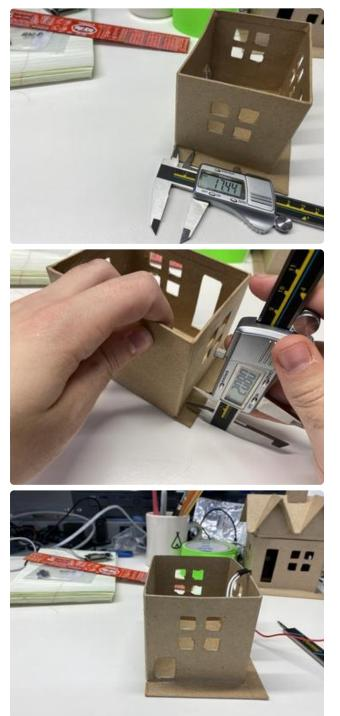
This portion is more tricky than it appears. The IOT House is made out of paper maché, not cardboard. If you cut this material slowly with a dull knife or scissors, it will de-laminate. You will want to use a very sharp X-Acto knife or something like the Slice Craft Knife which has a ceramic blade ().
