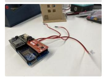
Before placing the Feather Huzzah32 and FeatherWings on the Quad FeatherWing, make sure that all the female JST connectors are routed through the middle and out the top of the Quad FeatherWing.
