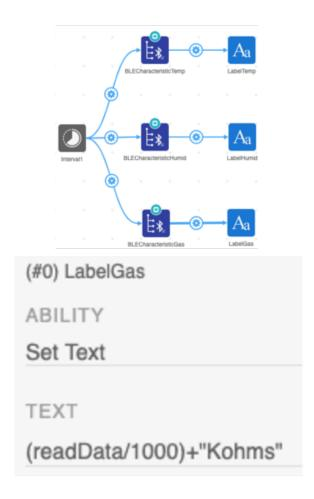
Finally, you'll set up the connection between the gas sensor reading and its label on the mobile application.
