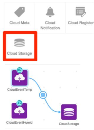
You'll need somewhere to send this data. Luckily, Digi-Key IoT offers up to 10 megabytes of cloud storage per device. To add data to this cloud storage, use the Cloud Storage Element.
