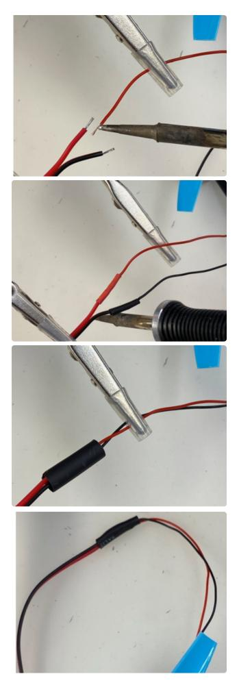
Using a soldering iron, tin the ends of both cables. Then apply heat with the soldering iron to connect them together.
