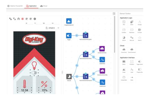
The Application Workspace allows you to design an interface to interact with your microcontroller from a tablet or smartphone. This workspace is split into two sides - a visual "App Builder" which allows you to drag and drop interface elements onto an application and a workspace for building the application's logic.
