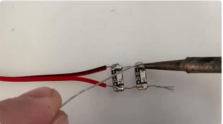
Add a second sequin to the chain, and solder it to the cable.
