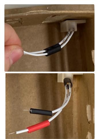
Strip 3mm of the rubber coating from the door sensor cable. Then, strip 3mm from the male JST header cable.
