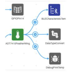
Add a new connector between the ADT7410FeatherWing Element and the DataTypeConvert element.
