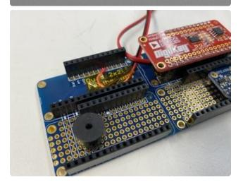
Place the buzzer on the prototyping grid. Make sure the buzzer's negative (short) lead is placed on the ground rail. Also, ensure the stacking headers will be able to fit besides the buzzer.
