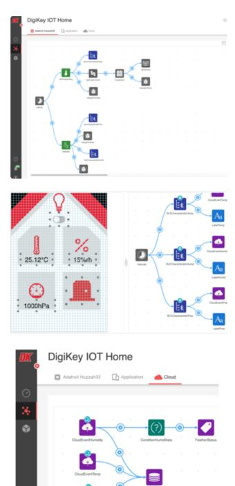
IoT projects involve programming firmware into a device, sending data from a device to "the cloud" and then interacting with the data and device using a website or application. Digi-Key IoT Studio comprises of three workspaces which simplify development:
