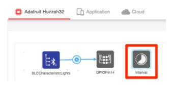
From the element toolbox within IoT Studio's Embedded workspace, click the Interval element.
