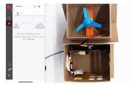
The fan will turn off after the temperature decreases below its target value.
