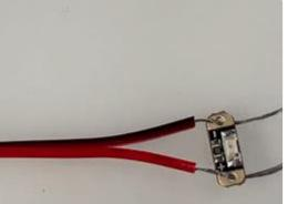
Using a JST cable with a male header, strip off a length of the rubber coating. Twist the stranded wire together and tin the bare wire using a soldering iron.
