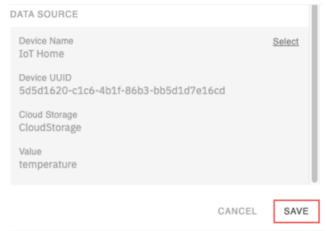
Select IoT Home as the device Select CloudStorage as the Cloud Storage Provider Select Temperature as the value Click Confirm to configure the data source. Then, click Save The gauge will automatically appear and the needle will move, reflecting the value read by your temperature sensor.
