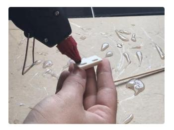
Using double sided tape or hot glue, affix the magnet to the door.
