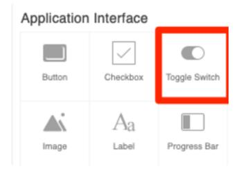
Digi-Key IoT Studio has an element which is perfect for controlling the lights in your home. The toggle Switch element is bidirectional and can be used to send either 1 or 0 to the lights to turn them on or off.
