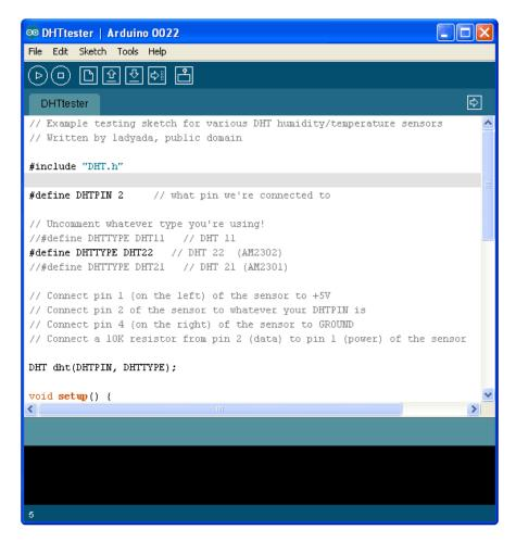
If you're using a DHT11 sensor, comment out the line that sets the type:
